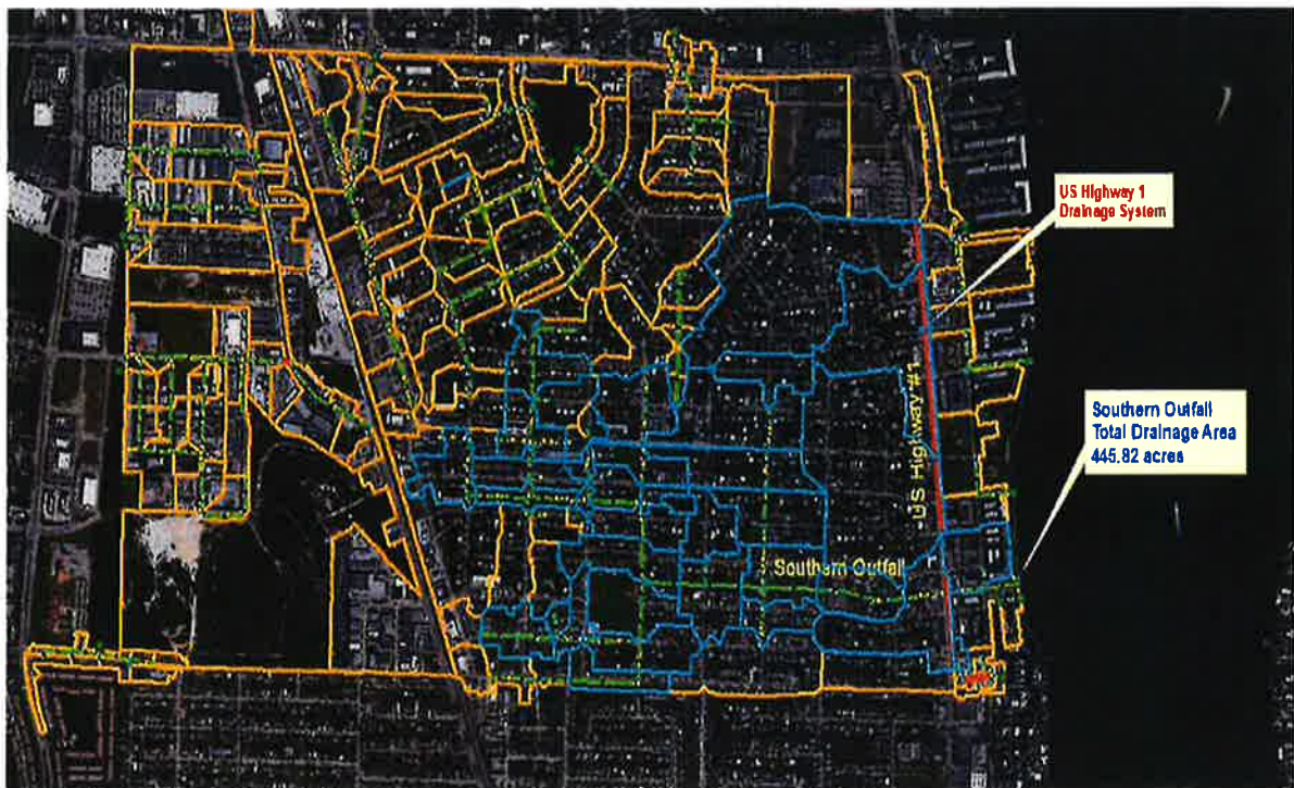
Figure 1. Southern Outfall and Drainage Area
