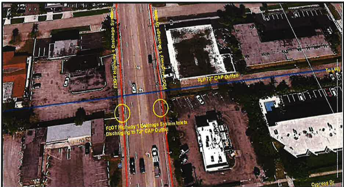
Figure 11. US Highway #1 Discharge Inlets at the 72" CAP Outfall
