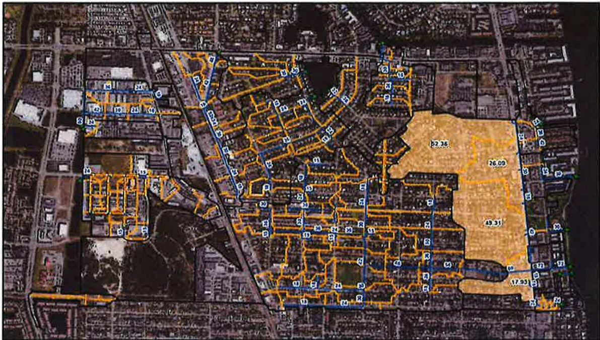
Figure 13. FDOT/US Highway 1 ROW Drainage Area Discharging to 72" CAP Outfall
