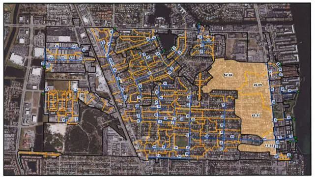
Figure 13. FDOT/US Highway 1 ROW Drainage Area Discharging to 72" CAP Outfall
