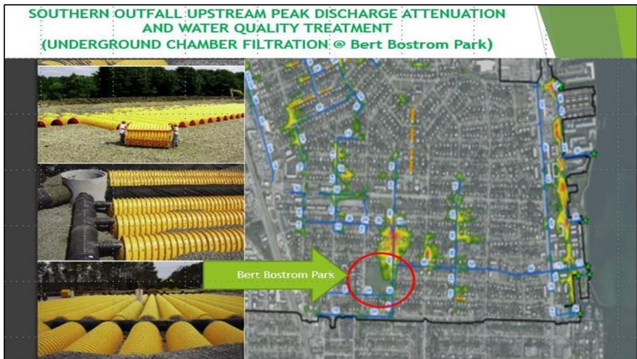
Figure 5-7 - Southern Outfall Diversion and GI Improvements
