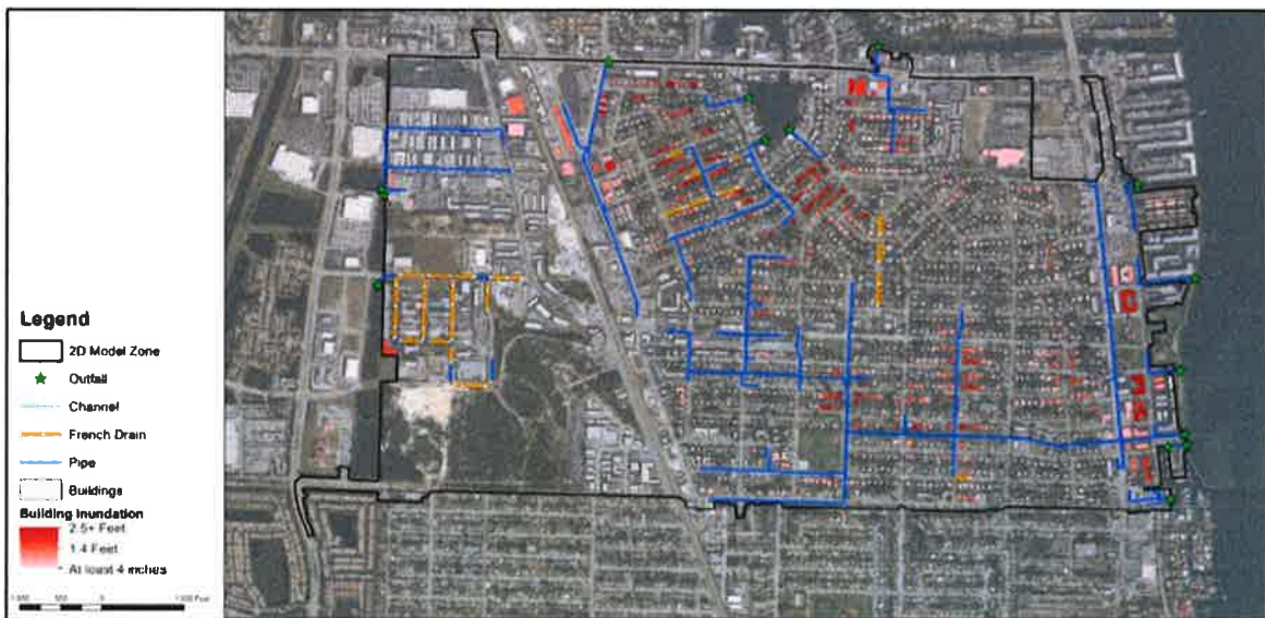
Figure 8-30 Structures Identified to be Flooded due to a 100-Year/72-Hour Storm Event
